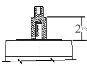
4. On JM style motors, apply Loctite RC/609 to inside diameter of shaft sleeve. Install shaft sleeve onto motor shaft making sure that the groove for the PTFE sleeve gasket is facing the pump end. Clean excess Loctite from shaft. Be sure sleeve is seated
