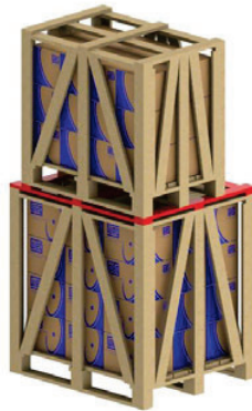
Figure 29 - Use of additional battens for stacking
