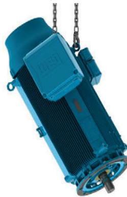
Figure 19 - Lifting HGF, W50 and W51 HD motors by the eyebolts at the non-drive end
