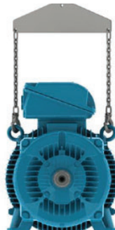
Figure 11 - Use of a spreader beam for lifting.
