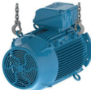
Figure 25 - Final result: motor placed in horizontal position
