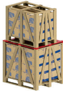
Figure 28 - Use of additional battens for stacking
