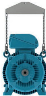
Figure 10 - Use of a spreader beam for lifting
