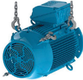
Figure 14 - Installation of the second pair of eyebolts
