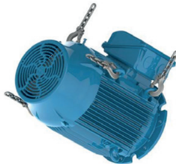
Figure 24 - Motor is being rotated to horizontal position
