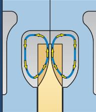
an MTH regenerative turbine, close internal clearances are required. In many cases, depending on the size of the pump, impeller to casing clearances may be as little as one-thousandth of an inch on each side. Therefore, these pumps are suitable for use only on applications with clean fluids and systems, or else the fluid must be pre-filtered before reaching the pump.
