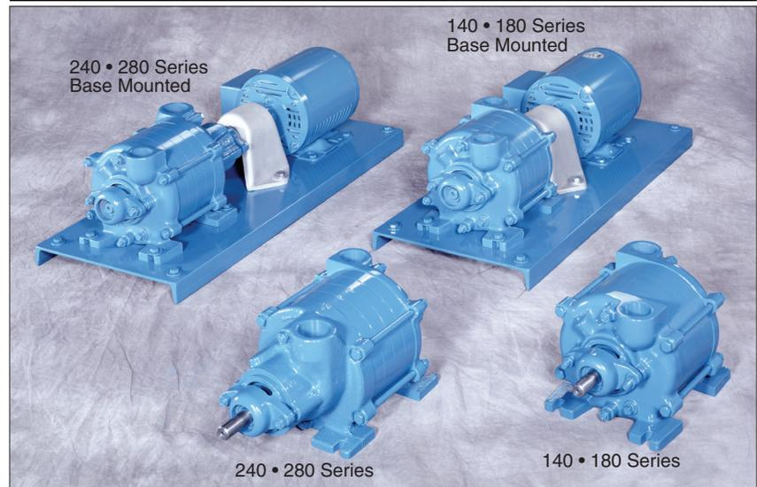
is cast bronze, hydraulically balanced and self-adjusting for longer life. Sealed ball bearings are permanently lubricated for maintenance free operation. "O" ring gasketing is used to assure sealing and for ease of maintenance. Standard mechanical seals are rated for 230°F water operation. All units are flexible-coupled for easy service and motor flexibility. Pumps are 100% tested to guarantee performance prior to shipment.
