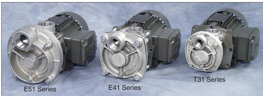
The **T31, E41, and E51 Series** close-coupled regenerative turbine pumps utilize our custom manufactured dual face 3450RPM D3 motors that incorporate a 304 stainless steel shaft and heavy-duty bearing. The stainless steel shaft eliminates the necessity of a shaft sleeve, thereby reducing the parts
