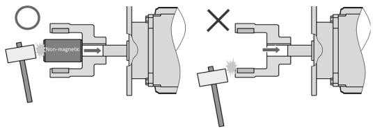
1-2 Press the magnet coupling straight onto the motor shaft. If it is at an angle, the shaft may be damaged.
