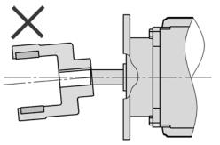
1-3 Press the magnet coupling in until the end of the motor shaft and the coupling (M) are at
