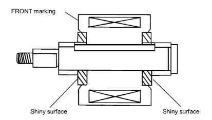
$\label{eq:cauchy} \textbf{CAUTION} \quad \textbf{\bullet} \ \text{When mounting the thrust ring, the shiny surface should be facing outside.}$
