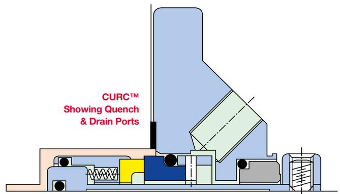
\*A version of the CURC™ can be supplied, with a fully machined gland, which conforms to the dimensional requirements of API 682. These can be used on applications where qualification tested, fully API 682 compliant seals are not required.
