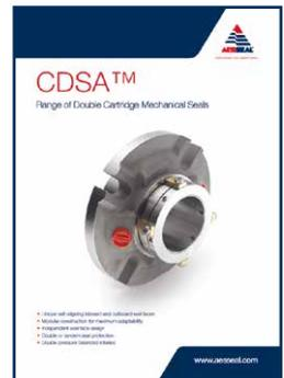
The CDSA™ has double pressure balanced rotaries and independent seal face design. It is also available with double or tandem seal protection. Both CURC™ and CDSA™ products employ modular components, thereby increasing availability and reducing product lead time.
