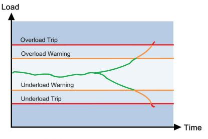
Emotron M20 shaft power monitor protects your pump and process against damage and downtime. Early warnings and trips allow preventative action to be taken.
