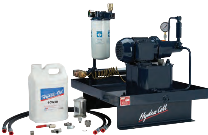
Water-cooled Oil Filter shown with complete kit.
