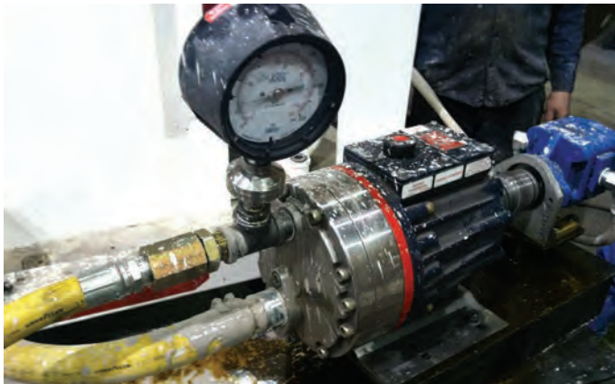
Pumping ceramic slurry in a spray drying application can be a problem for other types of pumps, but not Hydra-Cell.
