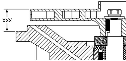
**Tighten all the setscrews after setting impeller clearance.**
