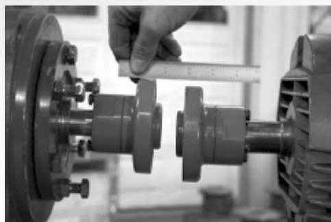
FIGURE 6 PARALLEL MISALIGNMENT
